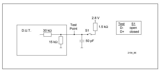
Figure 127 Load for D+/D-
