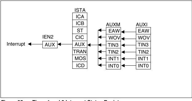
Figure 35 Timer 1 and 2 Interrupt Status Registers
