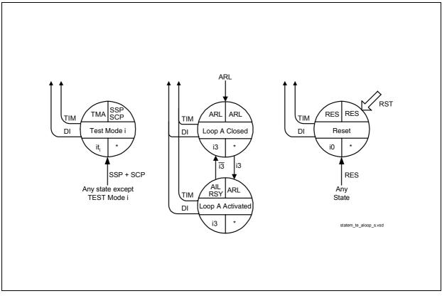
Figure 57 State Transition Diagram of Unconditional Transitions (TE)
