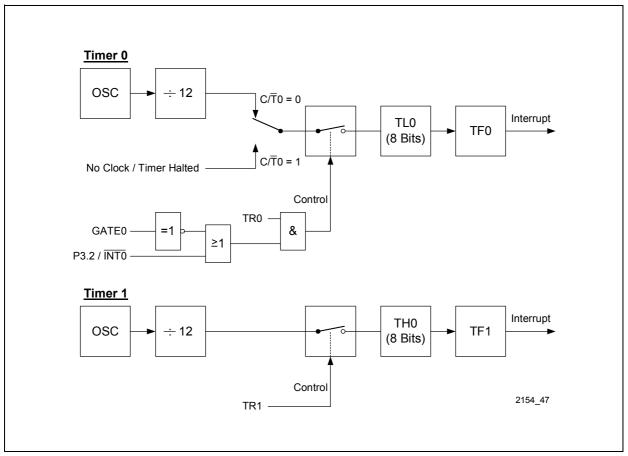
Figure 11 Timer Mode 3: Two 8-Bit Timers
