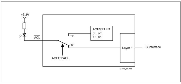
Figure 39ACL Configuration
