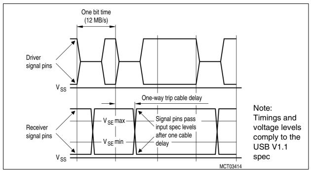
Figure 29 Full Speed USB Driver Signal Waveforms
