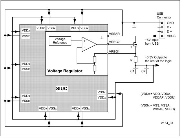
Figure 118 External Circuitry of the Voltage Regulator
