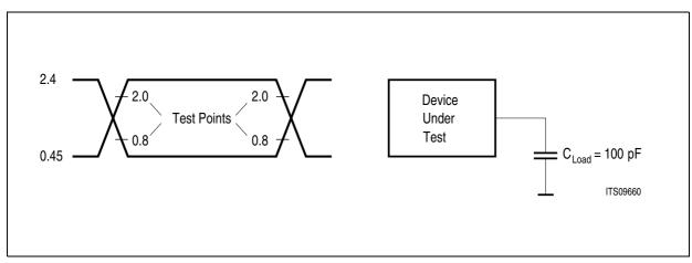
Figure 122 Input/Output Waveform for AC Tests
