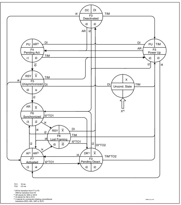
Figure 56State Transition Diagram (TE)
