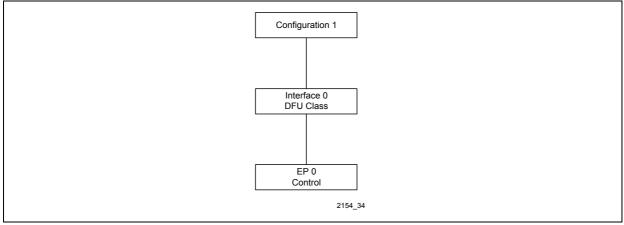
Figure 110 USB Configuration in DFU Mode
