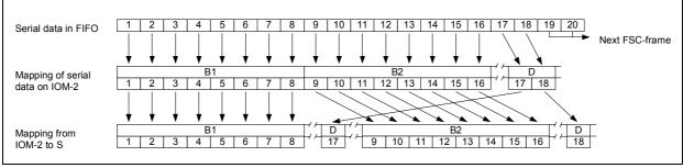
Figure 73 Mapping of Bits from IOM-2 to S
