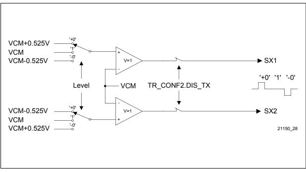
Figure 47 Equivalent Internal Circuit of the Transmitter Stage
