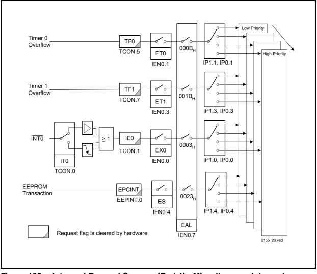
Figure 100 Interrupt Request Sources (Part 1) - Miscellaneous Interrupts
