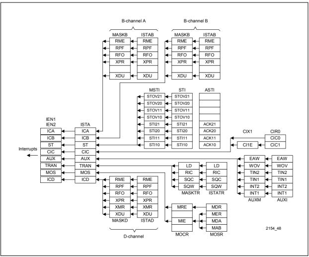
The structure of the ISDN interrupt status registers is shown in Figure 104.
