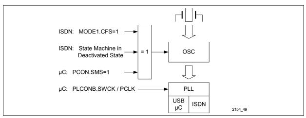
Figure 119 Clocks in Suspend Mode
