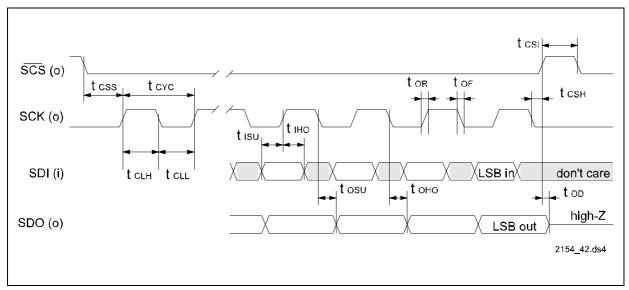
Figure 126 AUX Interface I/O Timing
