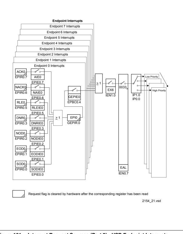
Figure 101 Interrupt Request Sources (Part 2) - USB Endpoint Interrupts
