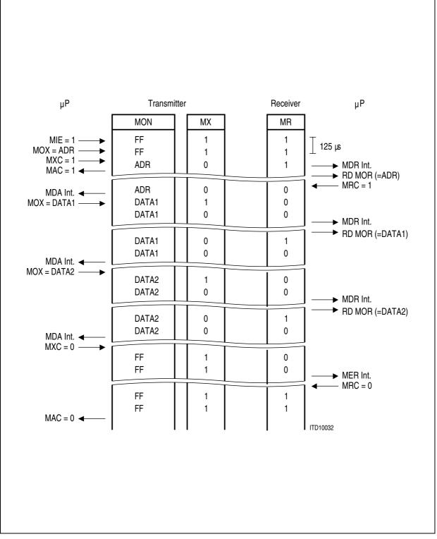
Figure 77 MONITOR Channel Protocol (IOM-2)
