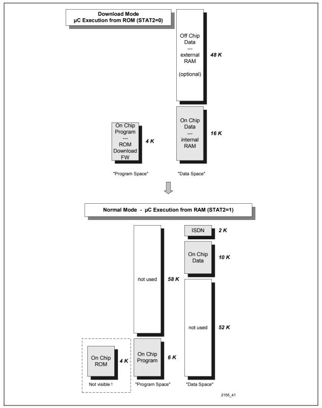
Figure 7 Switching from Download Mode to Operational Mode
