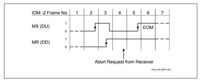
Figure 78 Monitor Channel, Transmission Abort requested by the Receiver
