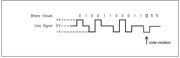
Figure 41 S/T -Interface Line Code
