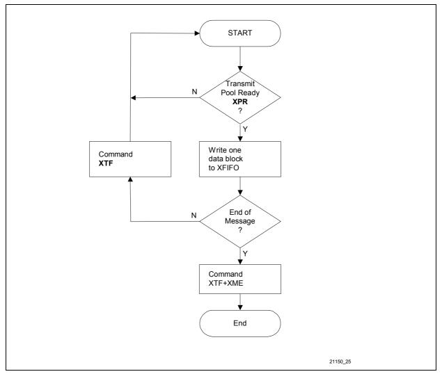
Figure 94 Data Transmission Procedure
