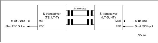
Figure 43 Multiframe Synchronization using the M-Bit
