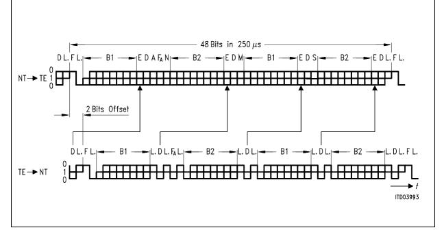
Figure 42 Frame Structure at Reference Points S and T (ITU I.430)
