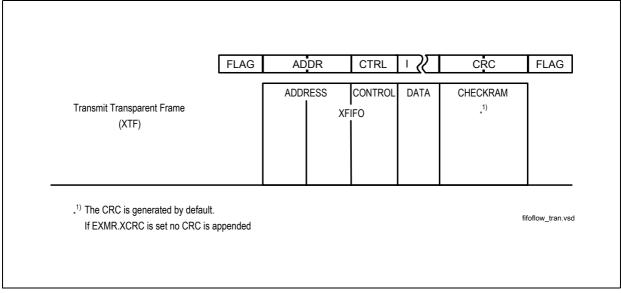
Figure 96 Transmit Data Flow
