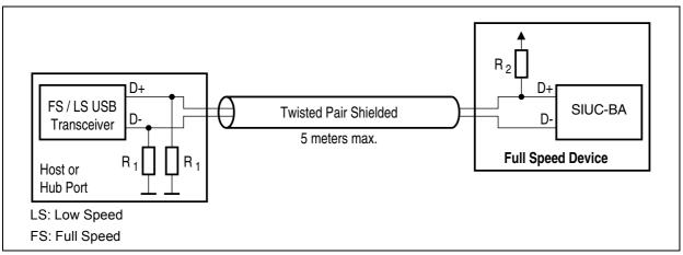
Figure 30 High Speed Device Cable and Resistor Connection
