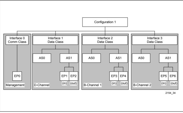
Figure 112 USB Configuration in CDC Mode
