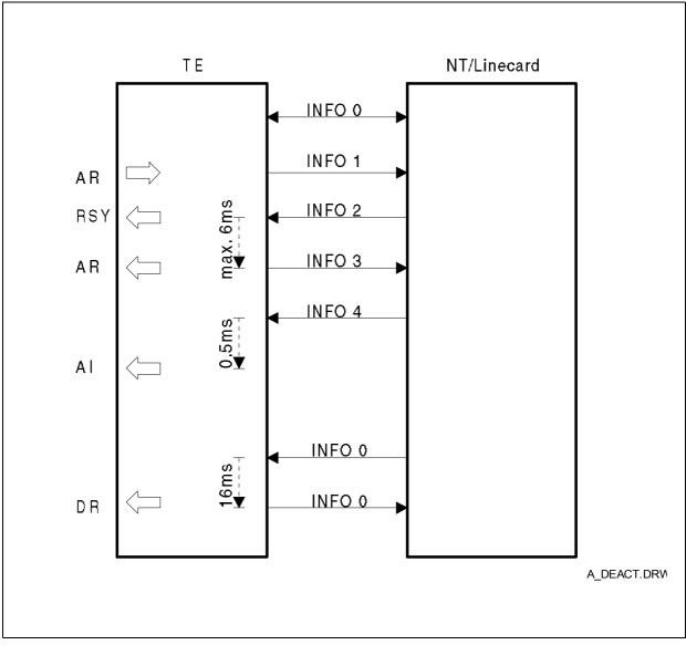
Figure 58 Example of Activation/Deactivation Initiated by the Terminal
