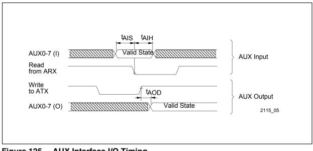
Figure 125 AUX Interface I/O Timing
