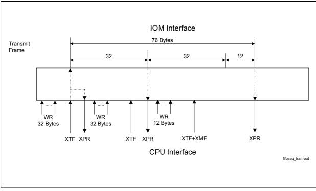
Figure 95 Transmission Sequence Example
