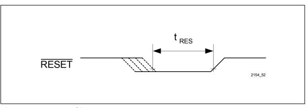
Figure 129 Reset Signal
