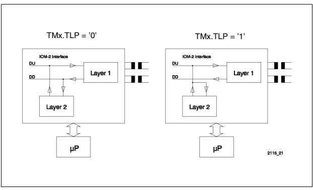
Figure 98 Layer 2 Test Loops
