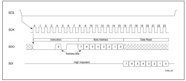
Figure 116 SPI Read Access
