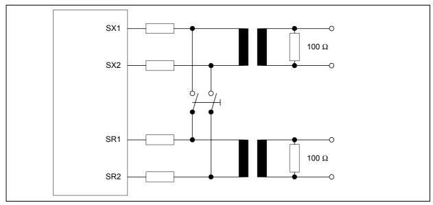
Figure 53 External Loop at the S/T-Interface
