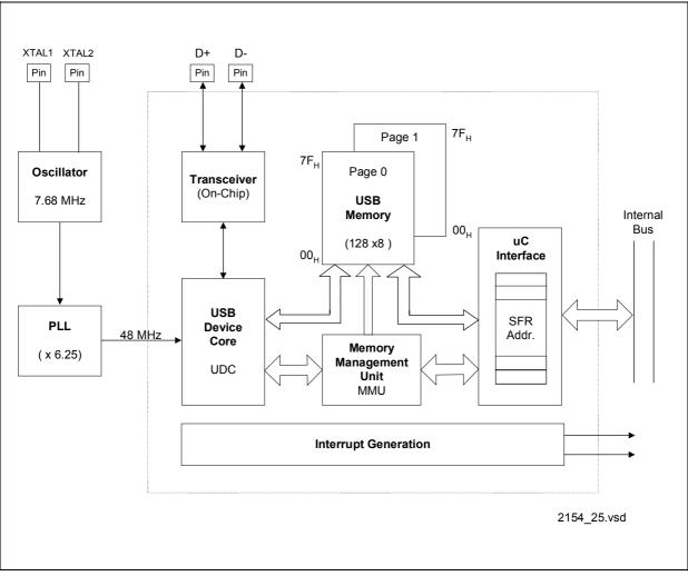
Figure 13 USB Module Block Diagram
