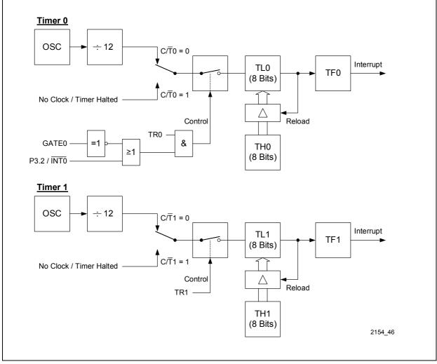
Figure 10 Timer Mode 2: 8-Bit Timer with Auto-Reload
