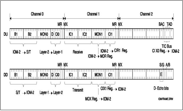
Figure 61 IOM-2 Frame Structure in Terminal Mode
