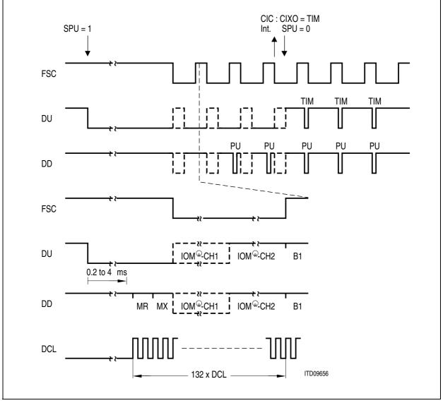
Figure 89 Activation of the IOM-2 interface
