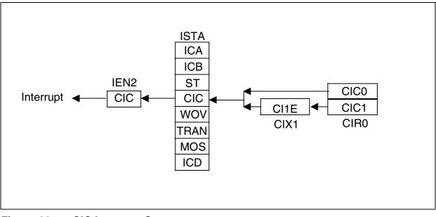
Figure 82 CIC Interrupt Structure
