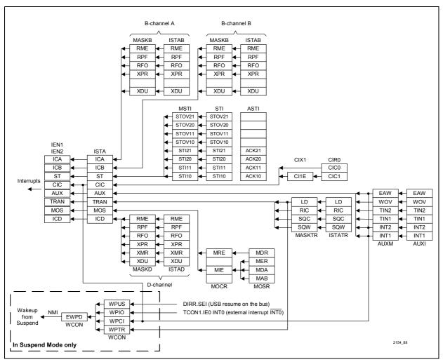
Figure 105 Wakeup Sources in Suspend Mode
