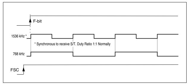
Figure 114 Phase Relationships of SIUC-BA Clock Signals
